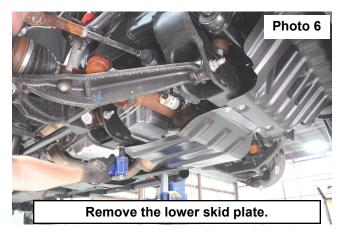
(For 2WD kits skip to step 14) 4WD Trucks, Use a 15mm socket, remove the lower skid plate. See Photo 6.
